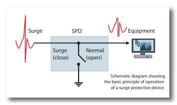
Fig 3 – When an overvoltage is detected the device begins to conduct
